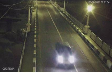
Example of poor installation for night conditions: the license plate is fully flared. The vehicle will be detected, but the license plate will not be recognized, although its presence or absence cannot be confirmed. Additional illumination is required.
