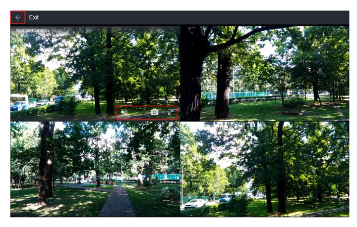
The buttons on the camera tile allow turning on/off the sound, save the frame to your computer and expand the video to full screen.
