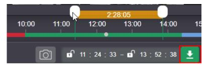
The button allows you to save the currently displayed frame of the archive in PNG format. The button is only displayed when current playback position is in the archive.
